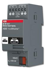
The device detects AC/DC signals of 10 - 230 V via 4 channels. The information of the signal evaluation can be used for controlling ABB-free@home® actuators or for recording status information. The bus can be connected via enclosed terminal block.
