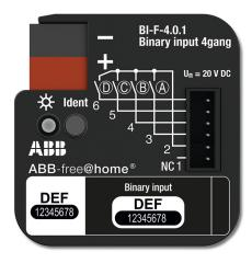
Conventional push-buttons or auxiliary contacts can be connected to 4 channels. The information of the contact enquiry can be used for activating ABB-free@home® actuators or for recording status information.
